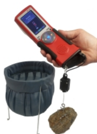
Density Measurement: Sample in Air
