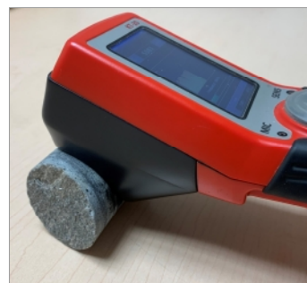
Curved Sensor Measuring Core Sample
