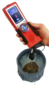
Density Measurement: Sample Submerged in Water
