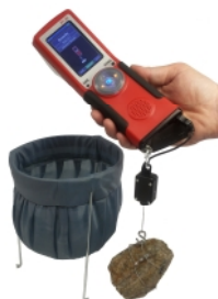
Density Measurement: Sample in Air
