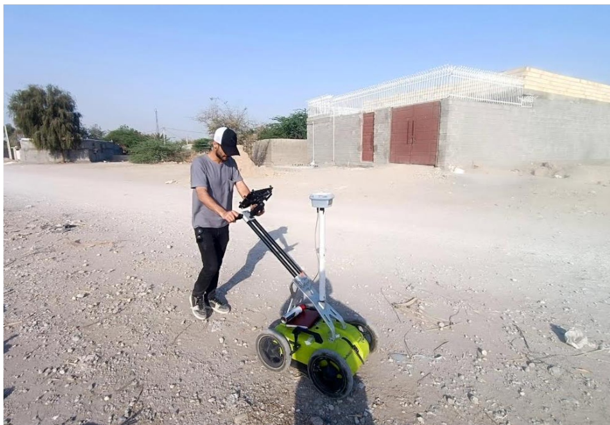
Figure 3 – Specialist conducting GPR data acquisition.
