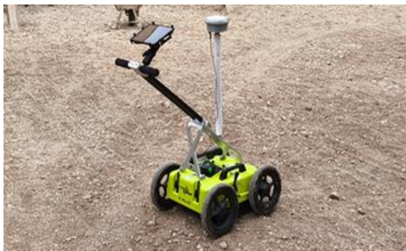
Figure 2 – ImpulseRadar PinPointR GPR device with multi-frequency GPS.
