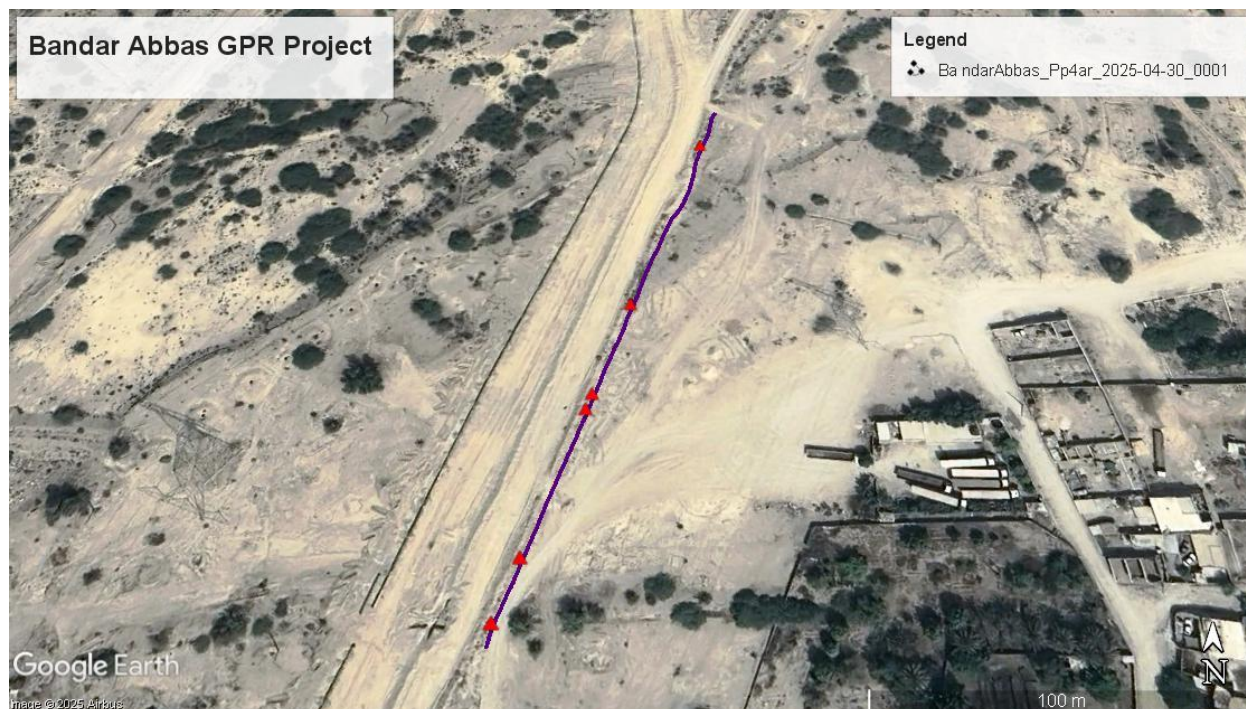
Figure 4 – Display of Profile No. 4 on the satellite image. The marked points indicate the locations of anomalies identified after initial data processing.
