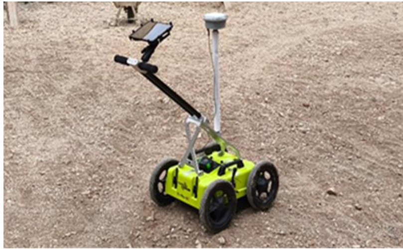
Figure 2 - The ImpulseRadar GPR device, PinPointR model, along with the multi-frequency GPS.
