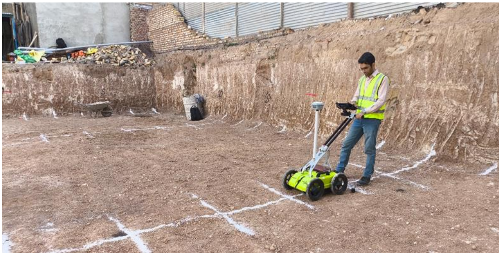
Figure 3 – Field Deployment of GPR System: field specialist conducts a grid-based GPR survey using the PinPointR dual-frequency antenna system ( ImpulseRadar ).
