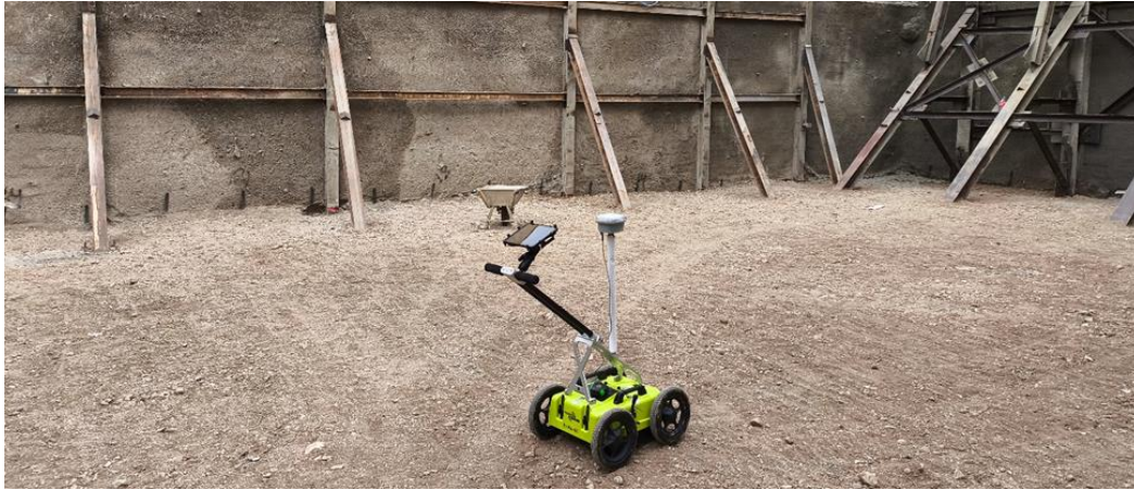
Figure 2 - The ImpulseRadar GPR device, PinPointR model, along with the multi-frequency GPS.
