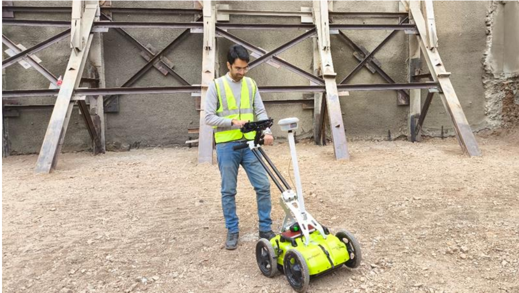
Figure 3 – Field Deployment of GPR System: field specialist conducts a grid-based GPR survey using the PinPointR dual-frequency antenna system ( ImpulseRadar ).
