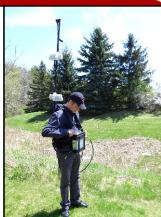
GEM Systems Overhauser Magnetometer system. It can be configured with additional survey sensors for simultaneous gradiometer readings as well as VLF. System configurations can also include walking mode and GPS.
