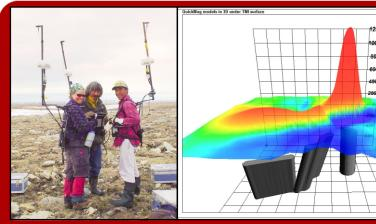
Single sensor and gradiometer modes provide flexibility and fast sampling and are used for detecting changes in the magnetic field. Applications include; alteration mapping, structural geology, archeology and UXO applications.
