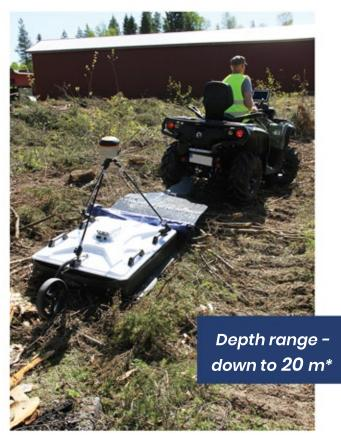
\*Figures for guidance only. GPR works best in high-resistive soils, absent of conductive layers. The actual depth range is dependent upon the di-electric properties of the ground or penetrable material under investigation.
