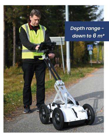
\*Figures for guidance only. GPR works best in high-resistive soils, absent of conductive layers. The actual depth range is dependent upon the di-electric properties of the ground or penetrable material under investigation.
