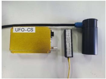
optical pumping magnetometer system complete weight: 1.5Kg (including battery)
