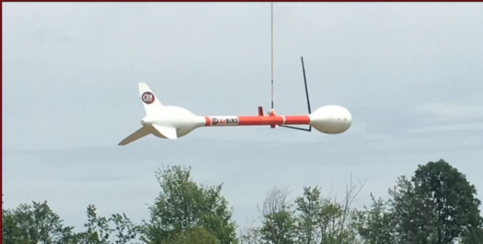
**The lightweight AirBIRD is a complete high sensitivity Potassium Magnetometer system for towing under an UAV. Complete with power, altimeter, GPS, data acquisition, data radio link, tow cable and ground control station.**
