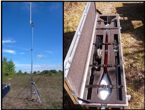
Radio Link ground station antenna and single case for complete storage and shipping.
