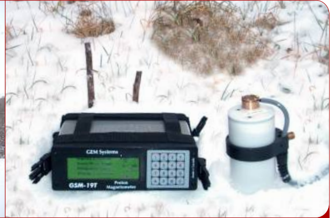
GSM-19TGW Proton Precession console configured with backpack, additional sensor for gradiometer (simultaneous) readings, built-in GPS and VLF EM system
