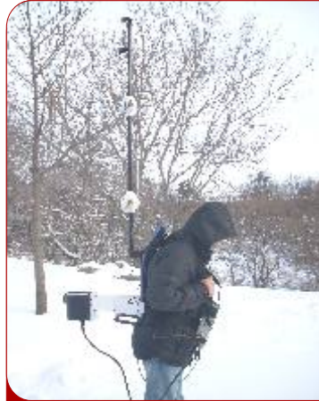
GSM-19TGW Proton Precession console configured with backpack, additional sensor for gradiometer (simultaneous) readings, built-in GPS and VLF EM system
