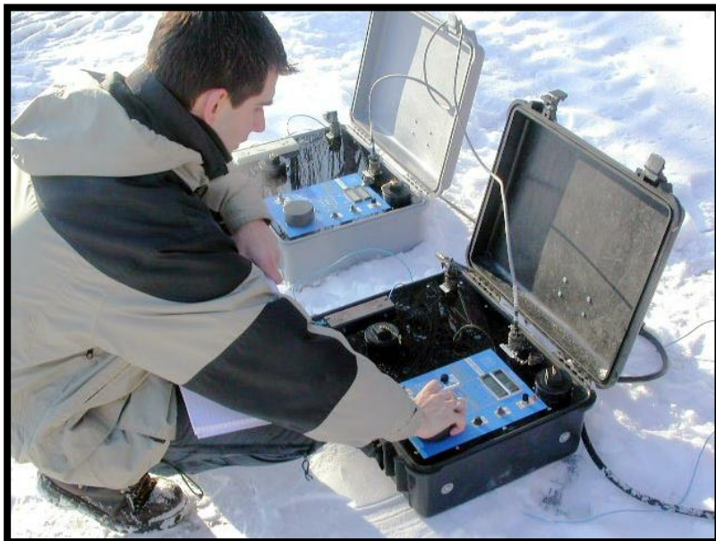
Model TxII in Master-Slave mode providing up to 10,000W-4800V-15A
