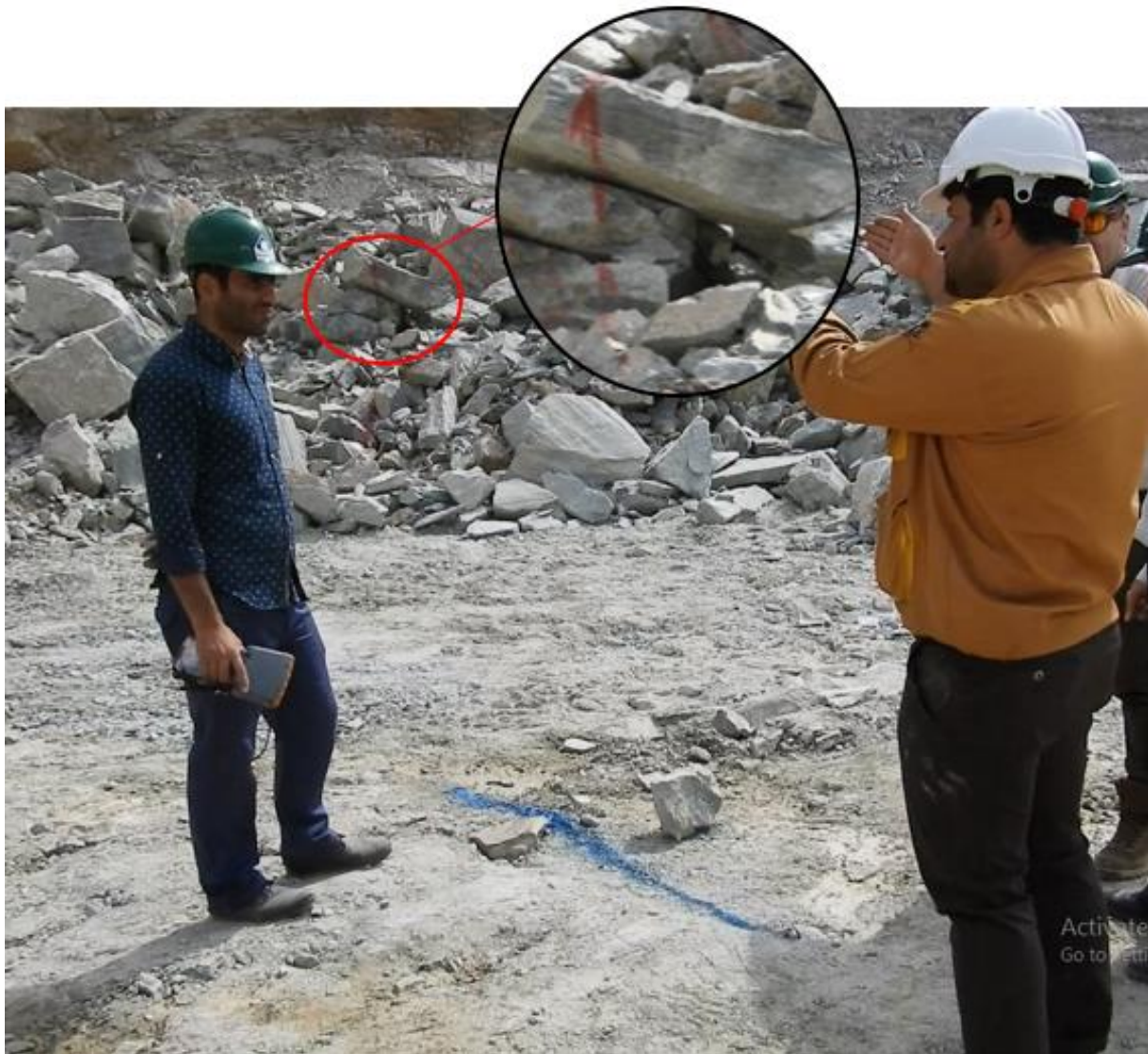
Figure 5. The result of IP survey (blue line) is compatible with the result of geological studies (red line)
